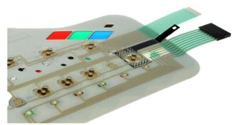
Heat stabilization allows the circuit printer to cure conductive inks at high temperatures with minimal effect on the registration or the lay-flat characteristics of the film.
